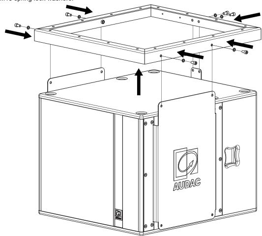
Attach the angle adjustment plates to the FX1.18 side plates using 4x ISO 4762 M10 x 20mm bolts and 4x DIN 7980 M10 spring lock washers.
