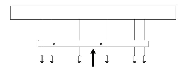
Slide the FX1.18 side plates around the frame and secure them with 6x ISO 4762 M10 x 20mm bolts and 6x DIN 7980 M10 spring lock washers.
