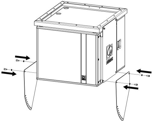
Slide the FX3.15 side plates between the angle adjustment plates and secure them in the right angle using 4x ISO 4762 M10 x 20mm bolts and 4x DIN 7980 M10 spring lock washers.
