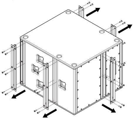
Mount the FX1.18 side and back plates to the FX1.18 cabinet and the FX3.15 side plates to the FX3.15 cabinet. You can use the bolts that were removed in step 1.
